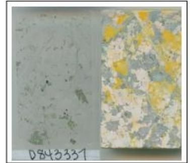
Sample of Fe-chlorite-epidote-sericite-altered granodiorite with magnetite (mt), where some mt crystals are being replaced by pyrite (py); from northeast of Boots.
