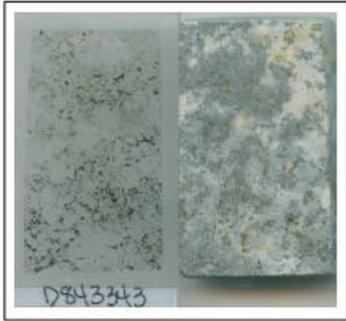
5.23% Cu in this pyrite-chalcopyrite-epidote-sericite-altered quartz diorite from Cu North.
